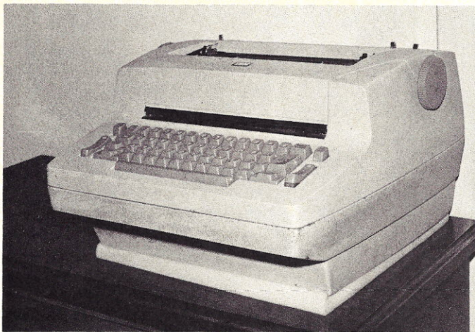
Photo 1. The IBM Model 731 Selectric as used in the 1014 Remote Inquiry Unit. The case has an extension on the bottom to house the solenoids, which permit remote operation of the typewriter.
